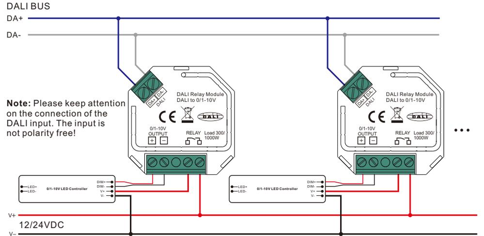
**Note:** the relay can also be connected to the input of the 12/24VDC PSU to switch 100-240V mains power.
